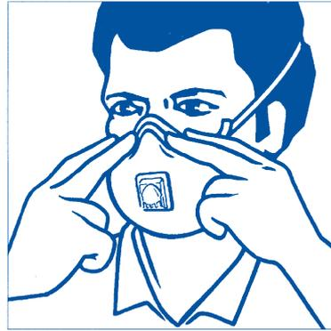
4. Place the fingertips of both hands at the top of the metal nosepiece. Mould the nosepiece to the shape of your nose by pushing inwards while moving your fingertips down both sides of the nosepiece. Pinching the nosepiece using only one hand may result in less effective respirator performance.
